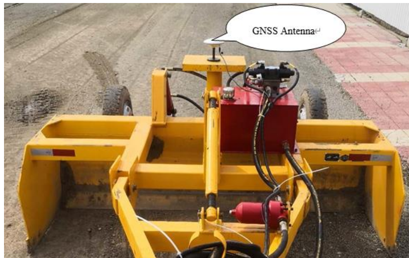
Figure 2.1 GNSS antenna installation
