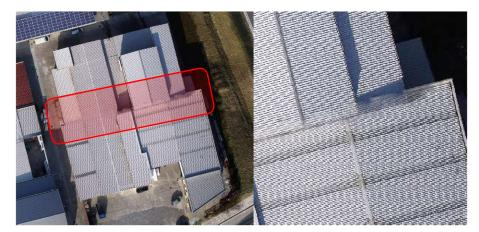
To eliminate the over-the-building image stitching we advise you to have the whole building on a single image. First, perform your mission at 80 m AGL, then manually trigger a few nadir images from a higher AGL (120 m above the object, for example) to get the whole object in one image.
