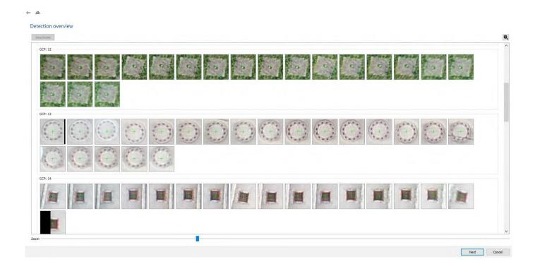
When you use Stonex targets the time needed to do the orientation will be much shorter. The possibility to do the mistake in choosing the target that is not correct is eliminated.
