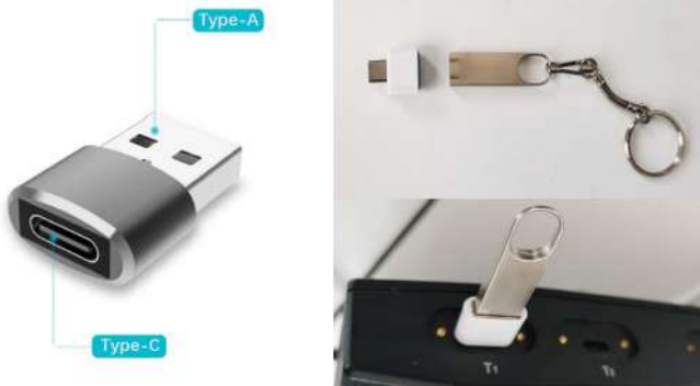
Figure 3.5.7 Connection diagram of mobile storage device
