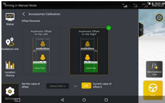
Figure 3.5.13 Settings for calibration of accessories
