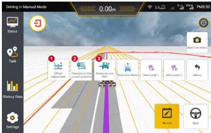
Figure 3.4.2 Selecting shifting method of guidance line
